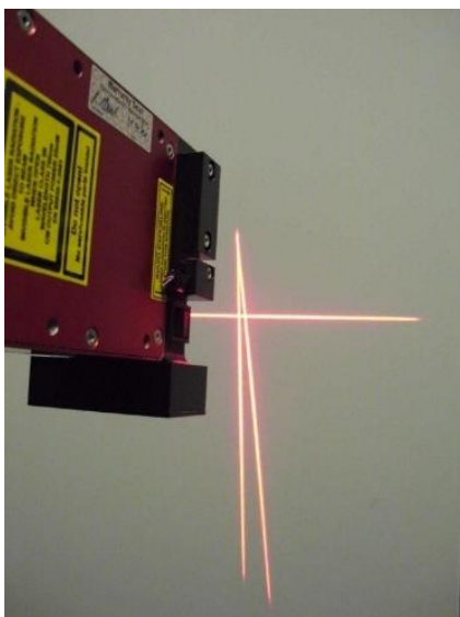
Figure 1: Sensor not vertical mounted
