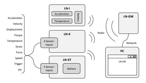
TEDIASENS systems are used for wireless measuring data transmission and data logging for industrial and geostationary applications. In addition to the TEDIASENS systems type SN-I and SN-X, used for synchronous data logging typically for short measurement times with online evaluation, there are now LOGGING NODE systems available for long-term monitoring with radio connection.
